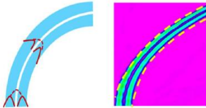
Fig. 3. Mode propagation at bending waveguide/region in proposing slit waveguide.
