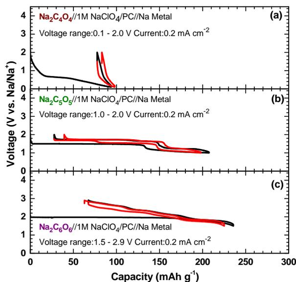
**Fig. 1:** Charge and discharge profiles of (a) Na<sub>2</sub>C<sub>4</sub>O<sub>4</sub>, (b) Na<sub>2</sub>C<sub>5</sub>O<sub>5</sub>, and (c) Na<sub>2</sub>C<sub>6</sub>O<sub>6</sub>, respectively.
