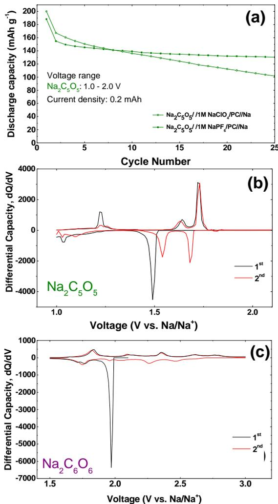
**Fig. 2:** (a) Cyclabilities of  $\text{Na}_2\text{C}_5\text{O}_5$  and  $\text{Na}_2\text{C}_6\text{O}_6$  in 1 M  $\text{NaClO}_4/\text{PC}$  and 1 M  $\text{NaPF}_6/\text{PC}$  electrolyte. dQ/dV curves of (b)  $\text{Na}_2\text{C}_5\text{O}_5$  and (c)  $\text{Na}_2\text{C}_6\text{O}_6$ , respectively
