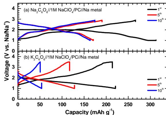
**Fig. 3:** Comparisons in charge and discharge profiles of (a)  $\text{Na}_2\text{C}_6\text{O}_6$  and (b)  $\text{K}_2\text{C}_6\text{O}_6$ .  $\text{Na}_2\text{C}_6\text{O}_6$  and  $\text{K}_2\text{C}_6\text{O}_6$  were cycled in 1.0 - 2.9 V and 1.0 - 3.5 V, respectively. The current density were  $0.2 \text{ mA cm}^{-2}$  in both cases.
