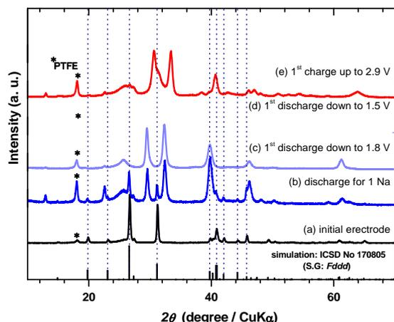
**Fig. 4:** *Ex-situ* XRD patterns of Na<sub>2</sub>C<sub>6</sub>O<sub>6</sub> at the state of (a) initial, discharge to (b) 1Na, (c) to 1.8 V, (d) to 1.5 V, and charge to (e) 2.9 V, respectively.
