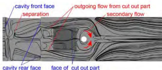
**Fig. 5:** Limiting streamlines on the duct lower wall.
