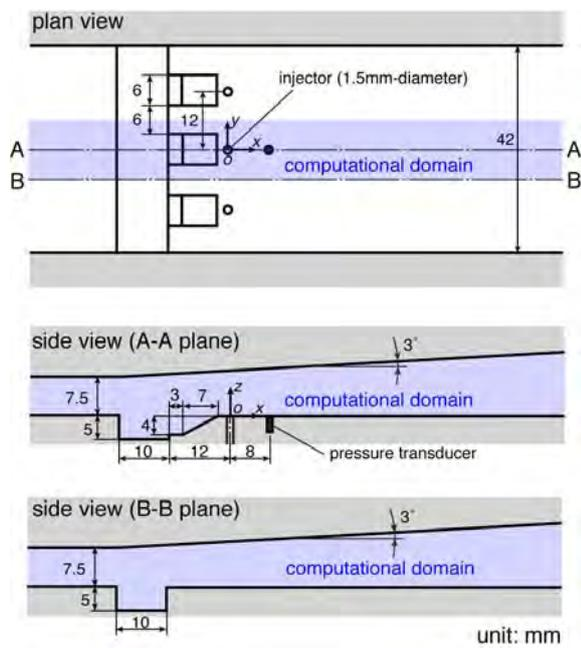
**Fig. 2:** Duct with the new device<sup>16)</sup>
