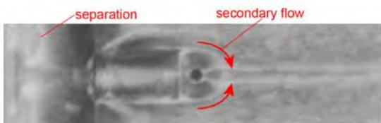
(b) duct with a three-dimensional cavity
