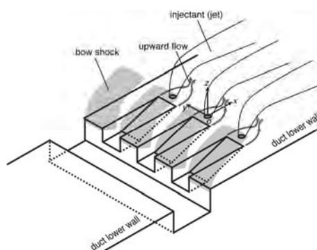
Fig. 1: New device for enhancing supersonic mixing<sup>16)</sup>.
