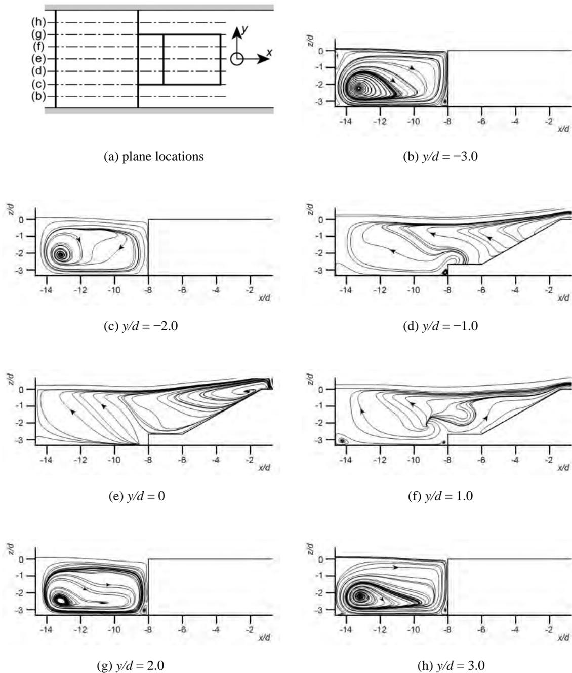
**Fig. 9:** Streamlines on the  $x$ - $z$  plane.
