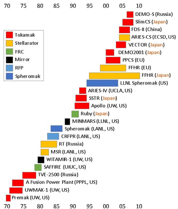
**Fig. 10.** Timeline of large-scale conceptual power plant designs developed worldwide for magnetic fusion<sup>16)</sup>.
