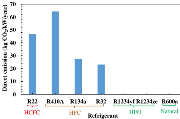
Fig. 4. Direct emission amount of CO<sub>2</sub> per kW/year from the residential air-conditioner.
