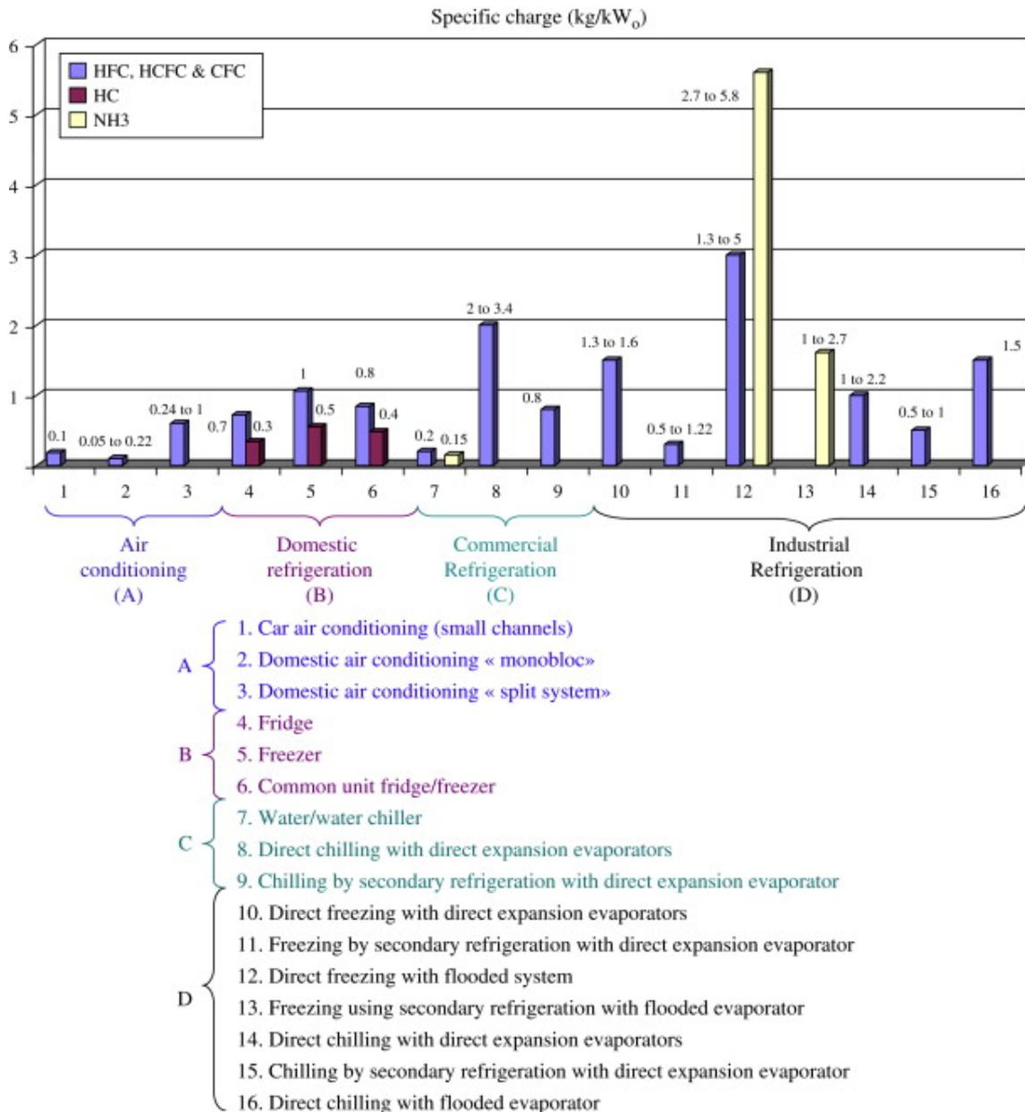
Fig. 3. Specific charge amount in complete systems for different applications using different refrigerants<sup>50</sup>.
