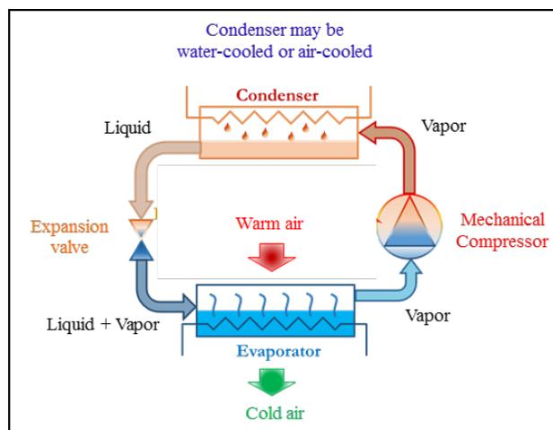
Fig. 1. Schematic diagram of a typical vapor compression refrigeration cycle<sup>17</sup>.
