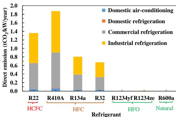
Fig. 5. Comparison of direct emission amount of CO<sub>2</sub> per kW/year from the various system.
