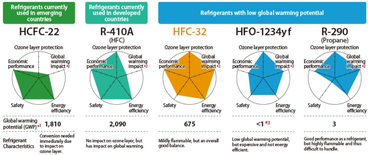
**Fig. 2.** According to Daikin, characteristics of possible next generation refrigerant for residential and commercial air conditioners<sup>38)</sup>. Here GWP values were reported according to IPCC 4<sup>th</sup> assessment report 2007 (AR4).
