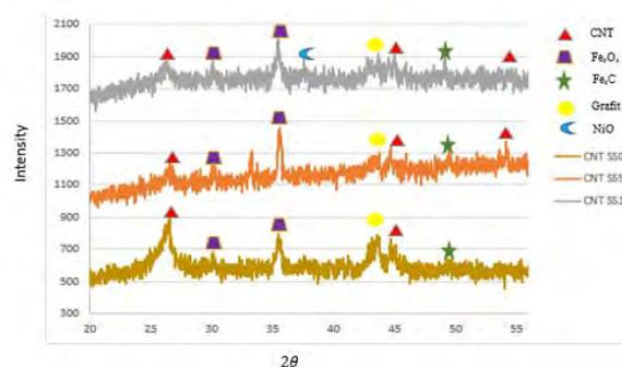
Fig 2. XRD Pattern of CNT samples
