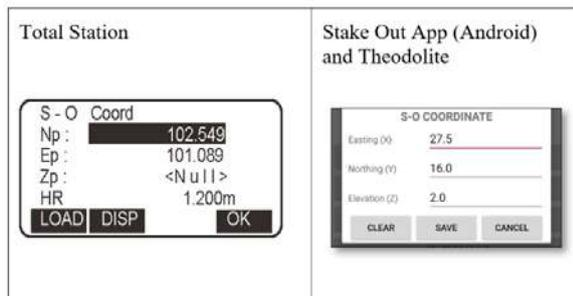
Fig. 6: Input Stake Out Data text.
