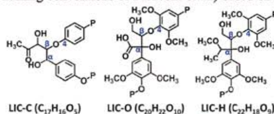
Figure 1. Reference dimer units in lignin structure. The solid residue start with P.
