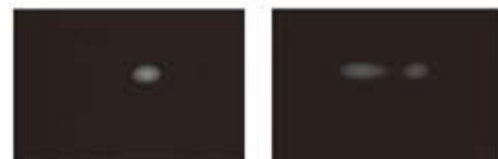
Figure 2. Near field pattern of (a) 0th mode (b) 1st mode
