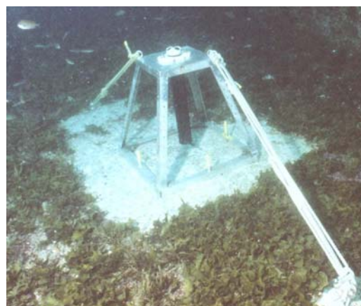
Fig.9 Photo of ADCP on the top of concrete caisson
