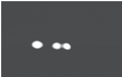
Fig. 9 Near-field-pattern of the fabricated novel active-MMI BLDs.
