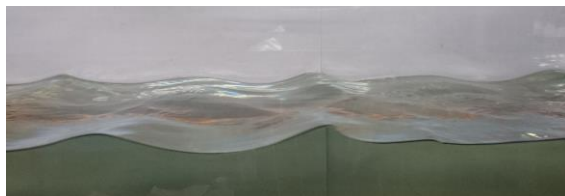
(c) U_r = 4.58 m/s ( U_{10} = 5.38 m/s, u^* = 0.081 m/s) [ MB ]
