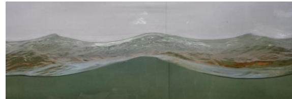
(d) U_r = 6.31 m/s ( U_{10} = 8.89 m/s, u^* = 0.223 m/s) [ B ]
