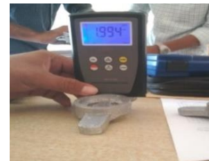
Fig.14:Cast part from ABS-Pattern(1.99µm)
