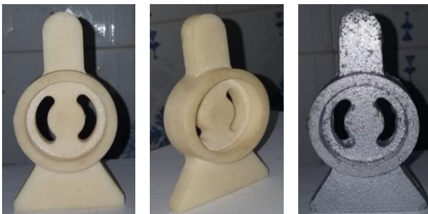
Fig.16: ABS-Patterns and Part from ABS-Pattern
