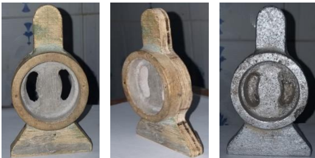
Fig.15: Wood-Patterns and Part from Wood-Pattern
