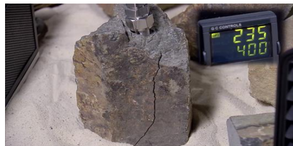
Fig. 5: Use of SMA to split the rock 102)
