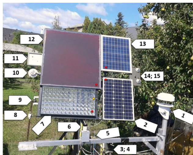
Fig. 1: Appearance and measuring instruments of the permanently installed measuring station capable of single- and dual-axis solar tracking according to 44,45 (1: DS-2 Sonic anemometer; 2: m-Si PV module; 3: HYTE-ANA-1735 humidity content of air meter; 4: JL-FS2 aluminum device with 3 spoons; 5: manual/automatic tracking control unit; 6: EMS 11 Silicon photovoltaic detector; 7: CPV module; 8: SN-500 four-component net radiometer; 9: photosensors; 10: Eppley Black and White pyranometer; 11: bracket mounted to detect angle change; 12: a-Si PV module; 13: p-Si PV module; 14: Hukseflux LP02 pyranometers; 15: EMS 11 Silicon photovoltaic detector; Orange dot: Pt 100 sensor in the CPV module; Blue dot: Pt 100 sensors at the bottom of PV modules)
