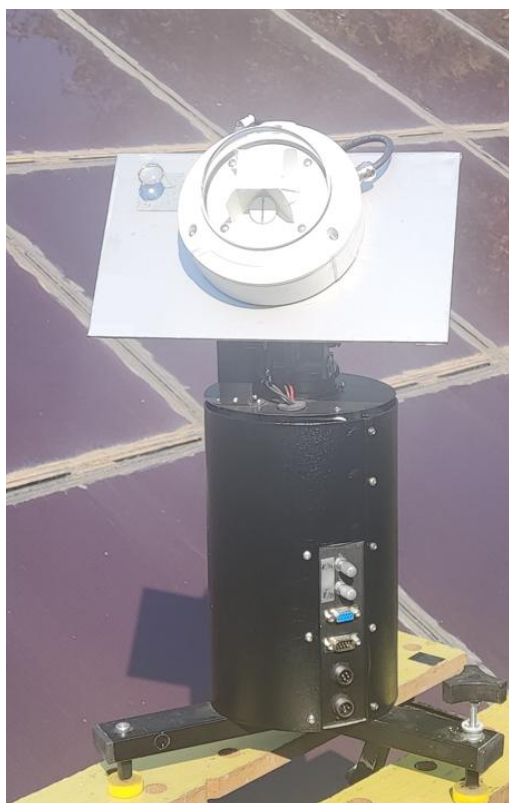
Fig. 7: Sensor control unit placed on the base of the designed mobile rotating mechanism for testing purposes, to determine the accuracy of the solar tracking
