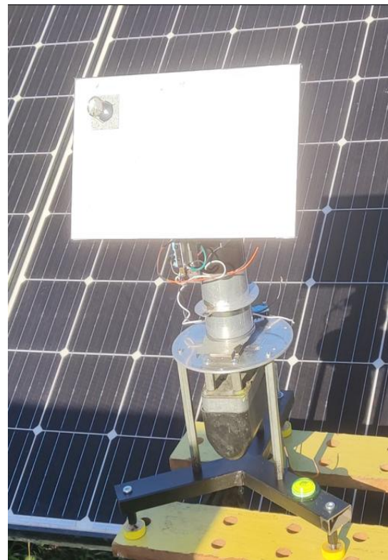
Fig. 5: The mobile rotation mechanism without electronics and casing with the base set in the south position
