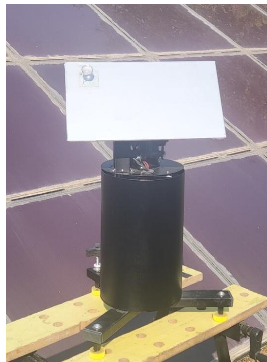
Fig. 6: The mobile rotation mechanism complete with electronics and casing
