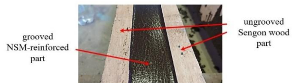
Fig. 6: Polymer concrete poured in the groove of timber or NSM-reinforced
