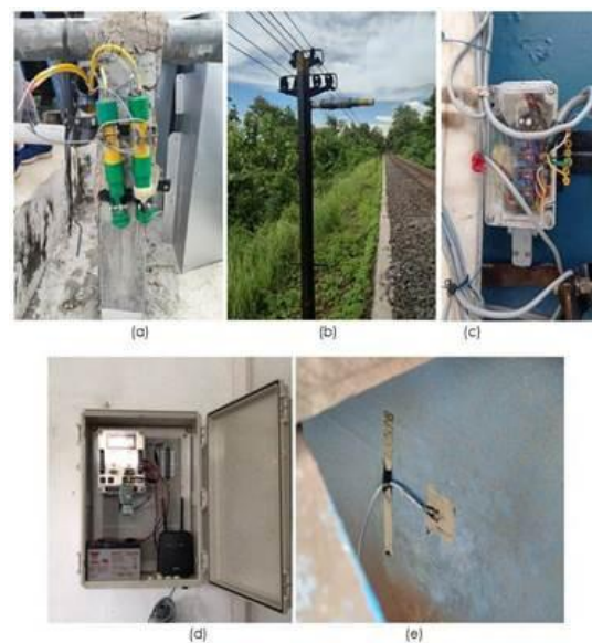
Fig. 5: (a) subsidence sensor; (b) PIR sensor; (c) modbus controller; (d) data logger; (e) strain gauge sensor
