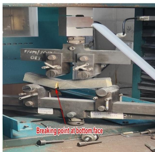
Fig. 15: Breaking point of carbon fiber (top 4 layers bottom 2 layers) sandwich composite
