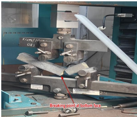
Fig. 12: Breaking point of carbon fiber (top 2 bottom 4) sandwich composite
