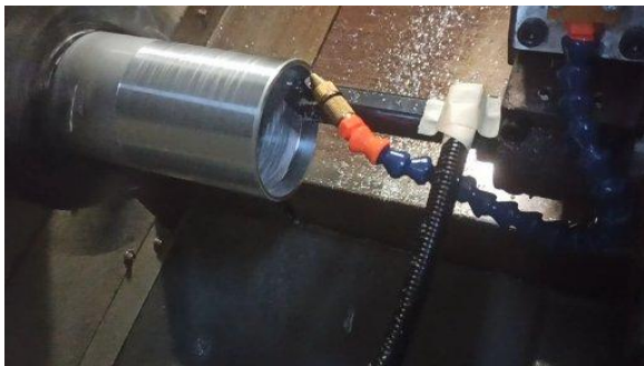
(b) Internal turning under MQL Fig. 2: Experimental Setup
