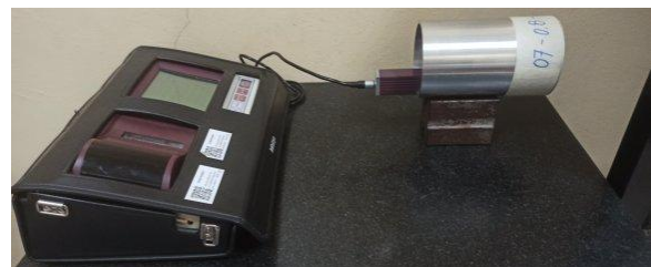
(b) SR measurement using Mitutoyo SJ-301 Fig. 5: Measurement Instrument
