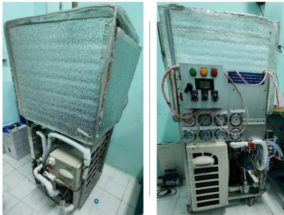
Fig. 2: Photos of R513A/R744 cascade system
