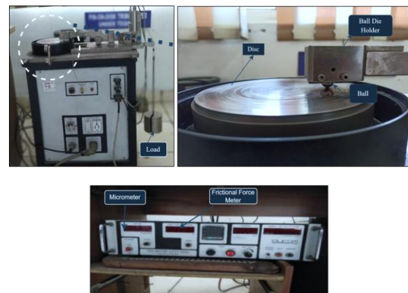
Fig. 1: Schematic of ball-on-disc wear test
