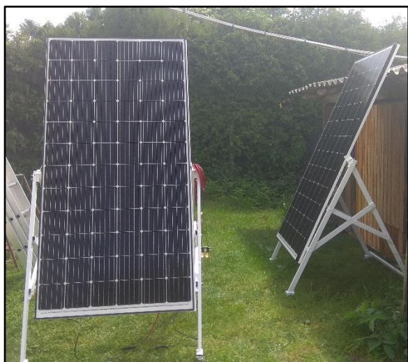
Fig. 1: Mobile mounting structure used for the investigation of the bifacial PV module
