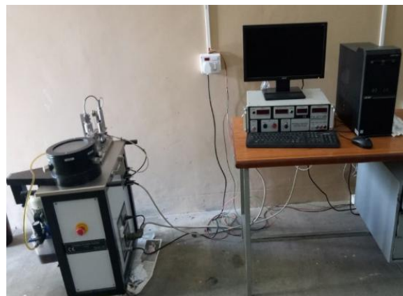
Fig. 1: Computerized Pin on Disc Tribometer Setup
