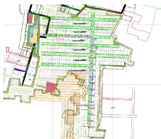
Fig. 7: Geometric representation of the main drainage channel used in the HEC-RAS hydraulic simulation
