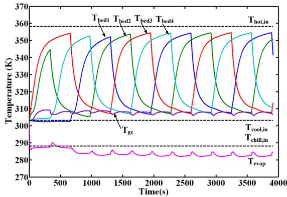
**Fig.2** Temperatures change of evaporator, gas cooler and the 4 beds of the simulated cycle.
