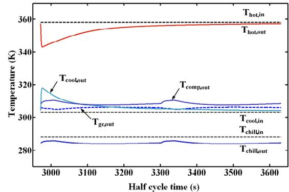
**Fig.3** Outlet temperature profiles during half cycle time.
