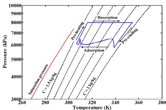
**Fig.4** *P-T-W* diagram of Maxsorb III-CO<sub>2</sub> thermal compression process.
