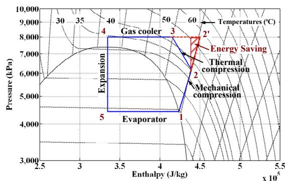
**Fig.5** *P-h* diagram of CO<sub>2</sub> based hybrid cooling cycle.
